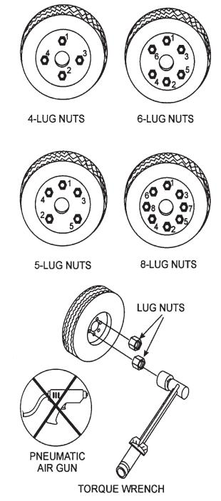
Figure 78. Wheel Lug Nuts Tightening Sequence
